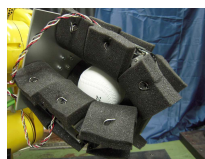
Fig. 10 Caging-based Grasping by a Multifingered Hand
