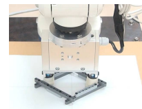
Fig. 11 Caging-based Grasping of a Deformable Object
