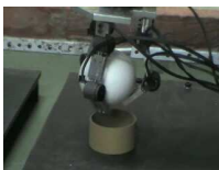
Fig. 9 Caging of a Sphere
