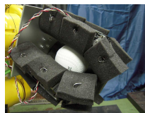
Fig. 10 Caging-based Grasping by a Multifingered Hand
