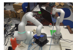
Fig. 19 A Robot System to Fold a Paper Crane
