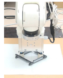
Fig. 12 Caging-based Grasping of a Deformable Object
