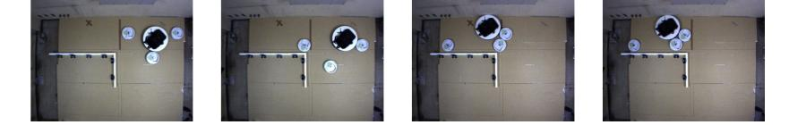
Manipulation by two circular robots with an RRT-based planner
