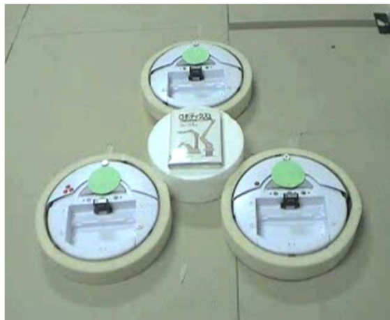
2D Grasping of circular objects by three circular robots
