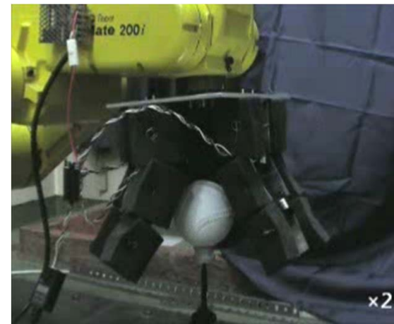
3D Grasping of spherical objects by a three-fingered hand
