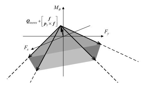
Possible Value of Q (contact forces + gravity) in Wrench Space
