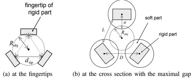
Fig. 11: Schematic views of the robot hand
