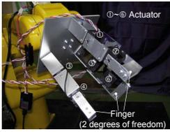
Fig. 12: Rigid parts of the hand
