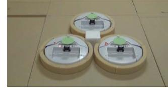
Fig. 16: Caging-based grasping of a rectangle
