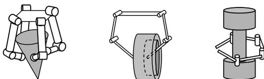
(a) Envelope-type caging (b) Ring-type caging (c) Waste-type caging
