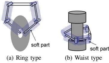
Fig. 8: Typical types of caging-based grasping
