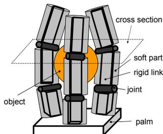
Fig. 10: A symmetric three-fingered hand
