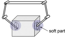
Fig. 9: Ring-type caging-based grasping using concavities
