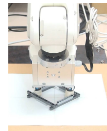
Fig. 12 Caging-based Grasping of a Deformable Object
