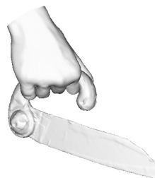
Fig. 23 A Synthesized Grasp of a Universal Design Knife by An Elderly Hand
