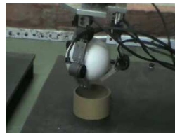
Fig. 10 Caging of a Sphere
